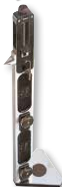
Using accessory items, gage blocks can be used to build height gages, snap gages, scribes and dividers. (Webber Heavy Duty style blocks are shown)
