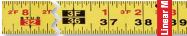
Quick-reading figures on a steel tape eliminate confusion and errors. Foot figures in red plus red foot figures before every inch mark. Red flag every 16 inches shows stud centers (Inch reading).
