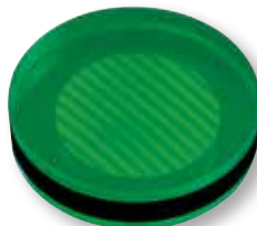
Fused quartz optical flats provide a quick, extremely accurate means of checking flatness of lapped surfaces.
