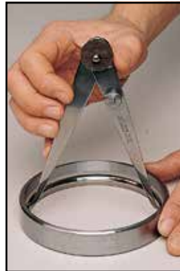
When holding contact measuring tools lightly by the fingers, it is possible to "feel" extremely slight differences in dimension.
