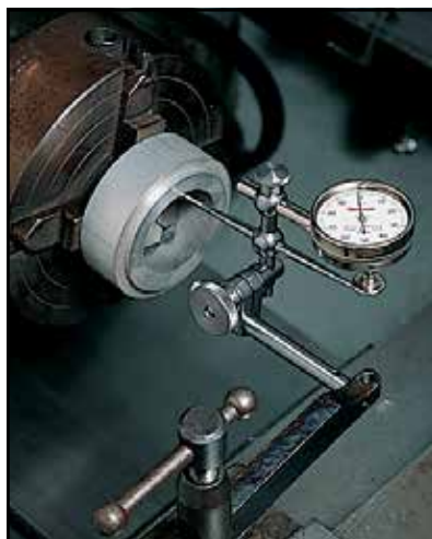
Checking lathework with dial test indicator. Tool post holder holds indicator securely in position.
