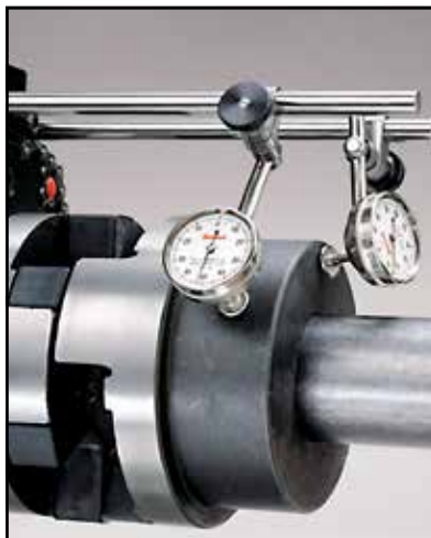
Starrett 196 Indicators check radial and angular alignment.
