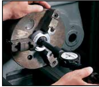
Bore measurement with a 84 Dial Bore Gage
