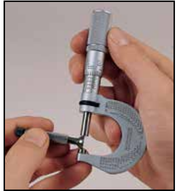
Starrett friction thimble micrometers (illustrated) and ratchet stop give uniform contact pressure for correct readings every time, independent of "feel".
