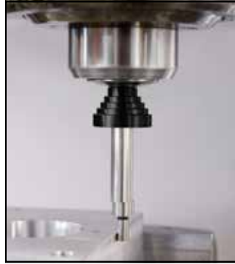
Locating work from straight edge using a single end edge finder mounted in chuck of machine tool.
