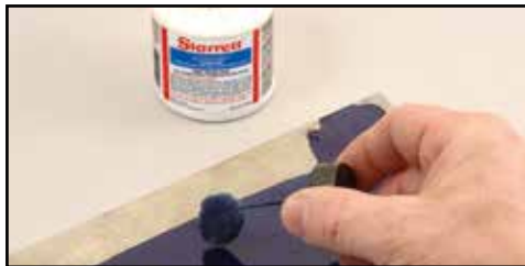
Blue layout dye being applied by brush.
