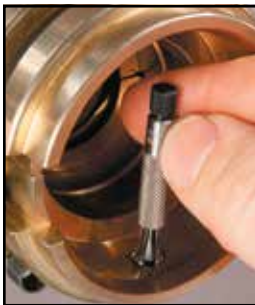
Ball contacts with flat ends allow shallow slots and recesses to be measured. Shown No. 830.
