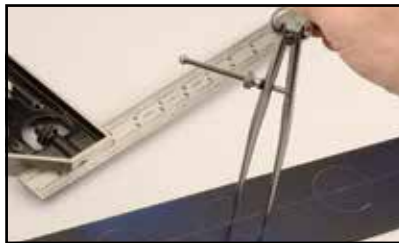
For precise layout of three identical circles, this mechanic uses 6" spring dividers.
