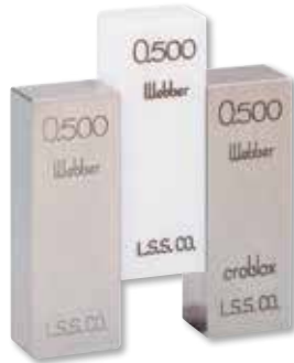
Gage blocks are primary standards with accuracies to a few millionths of an inch.
