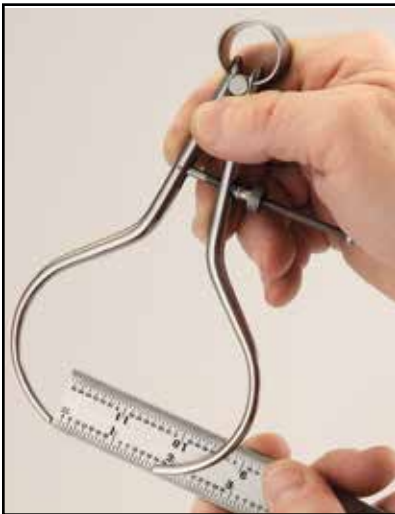
Pre-setting outside calipers to a rule for a transfer measurement.
