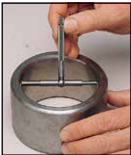
Accurate measurements are ensured with telescoping gage. Handle is automatically self-centering. Shown, No. 579.
