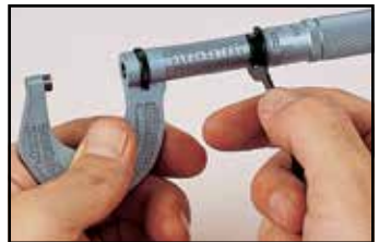
Illustrated: Adjusting spindle play.
