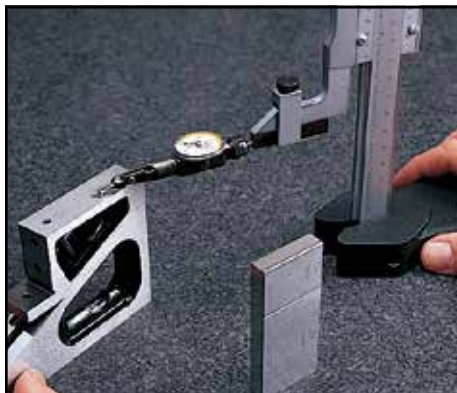
Last Word® dial test indicator attached to Vernier height gage for comparing measurements from gage blocks with the work. Shown with the PT99441 attachment that allows using many dial indicators.
