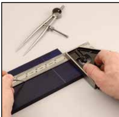
Scribing right angles and parallel lines using a combination square.
