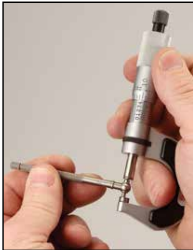
After establishing hole size with a telescoping gage, actual size is determined by measuring over the contacts with an outside micrometer.
