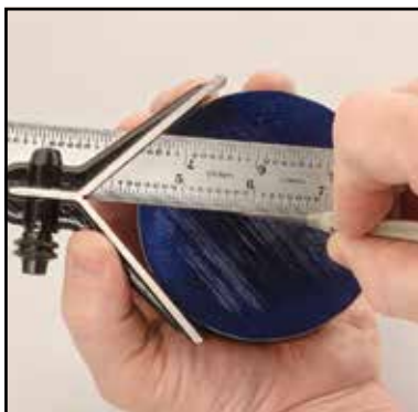
Center of round work can be accurately determined using the center head of the combination square.
