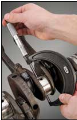
Measuring round work, a crankshaft journal, with an outside micrometer.
