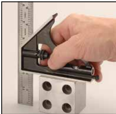
The combination square used as a depth gage. A very handy application.
