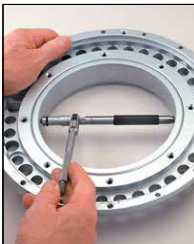
Checking inside diameter of a deep hole with an inside micrometer. Convenient handle is attached to the center of the micrometer.
