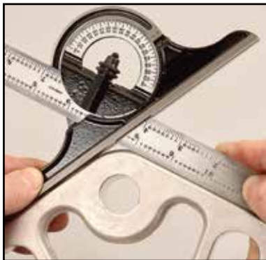
The protractor head on a combination set accurately and quickly checks angles.
