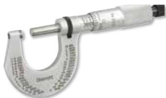
Ratchet stop on micrometer ensures consistent gaging pressure.
