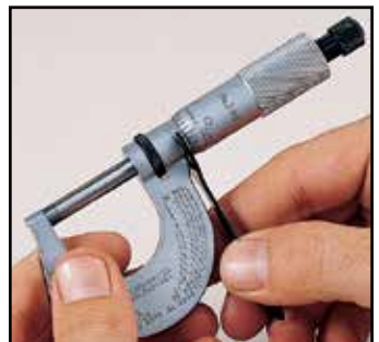
Illustrated: Adjusting for zero reading.
