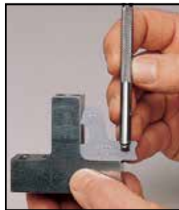
Radius Gage in holder provides fast check of 1/4" radii milled on this work piece. Shown No. 167 with a No. 110 holder.
