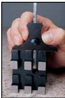
Checking the depth of a blind hole with a depth gage.
