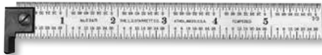
Starrett H604R-6 Spring Tempered, 6 inches long. Graduations in 8ths, 16ths, quick reading 32nds and 64ths. The single hook is hardened and may be reversed or removed entirely by a slight turn of the eccentric stud.
